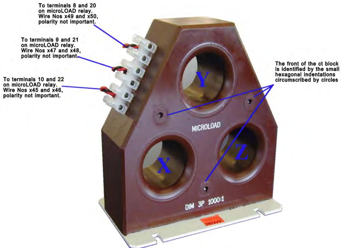
The single phase voltage transformer that supplies the microLOAD relay must derive its power from the phases that pass through holes X and Y.
