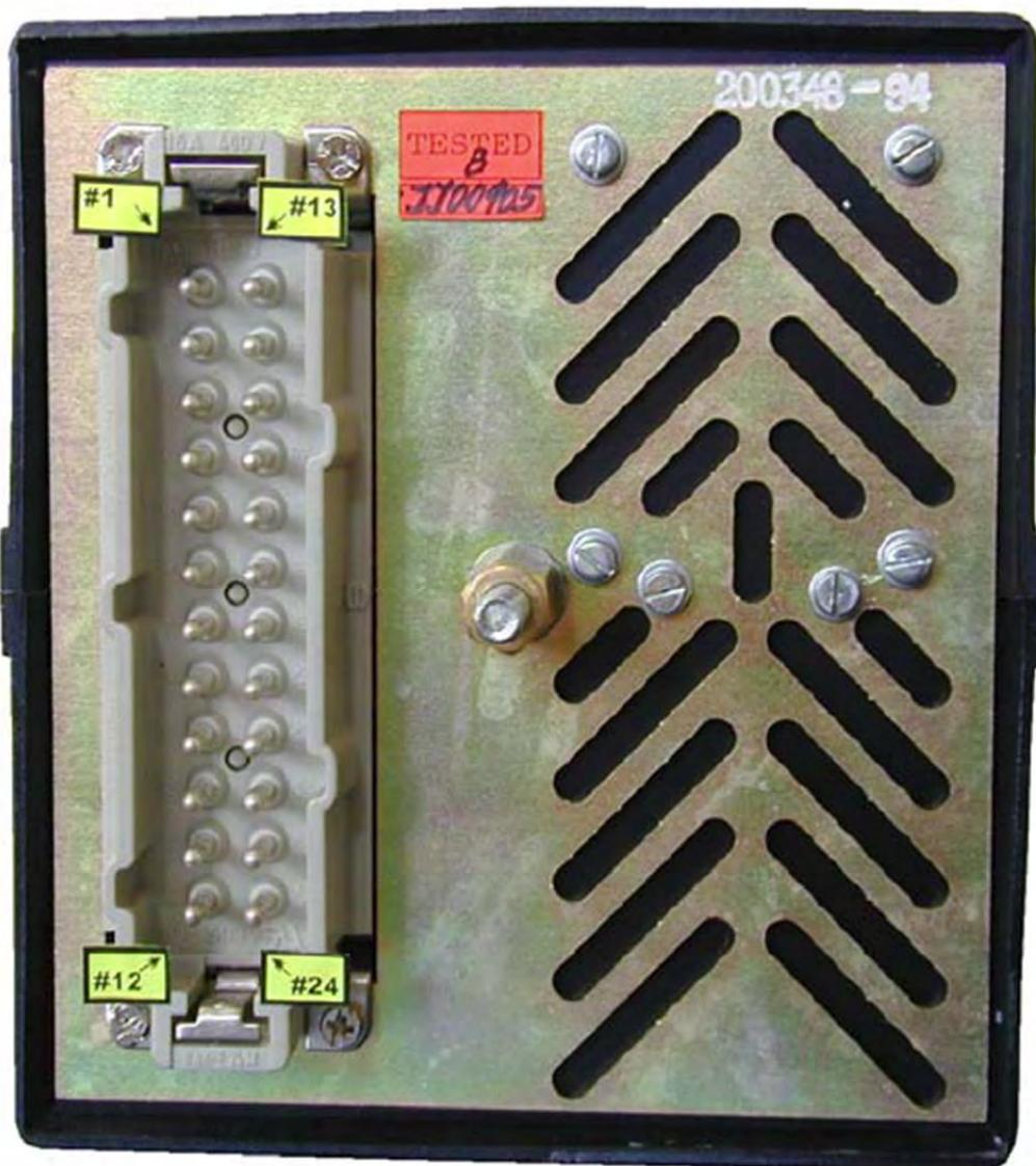
**Figure 2: The rear terminal layout of the microLOAD Relay**
