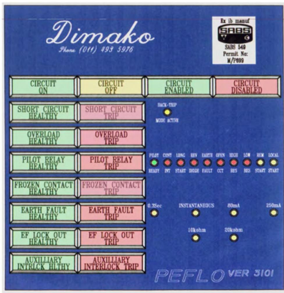
**Figure 1: The general layout of the front panel of the PEFLO protection relay**
