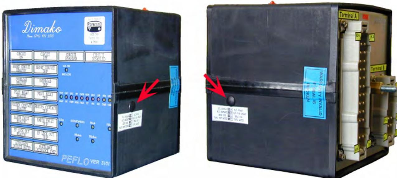
**Figure 2: The location of the parameter setting switches on the side of the PEFLO Relay**
